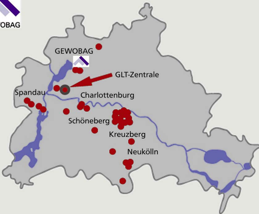
76 GEWOBAG properties are currently connected. The MPLS network can be routed cross-regionally via tunnelling.
